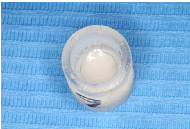
Figure 2: PEEK disks embedded in epoxy resin
