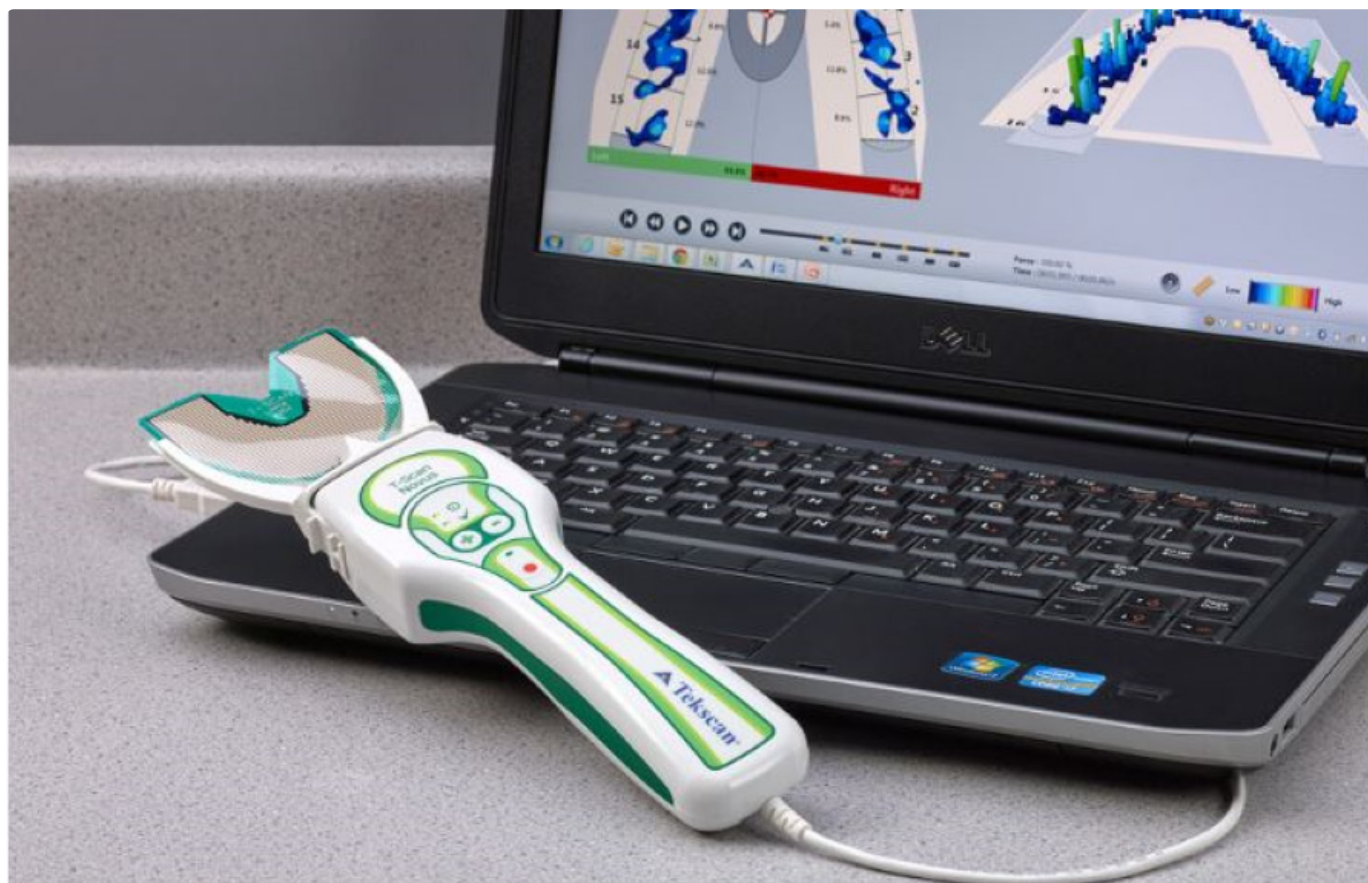
Figure 3: The T-Scan 10 Novus recording handle loaded with a Novus HD sensor, that is connected via USB to the T-scan 10's companion, color-coded force and timing software
