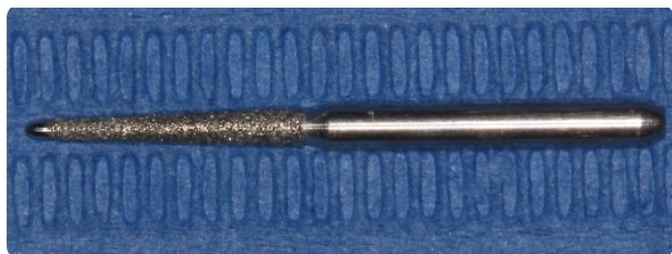
Figure 1: Komet 857 314/014 bur, showing the non-cutting tip which ensures the base of the sulcus is not violated
