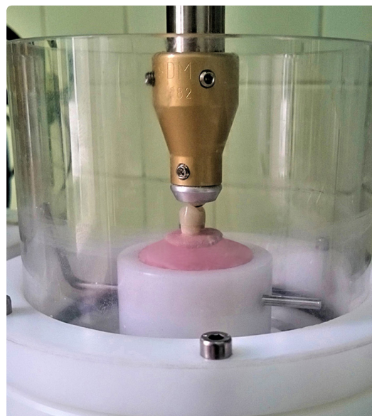
Figure 6: Dynamic Loading Testing; the specimen in its chewing simulator position with centralized axial loading.
