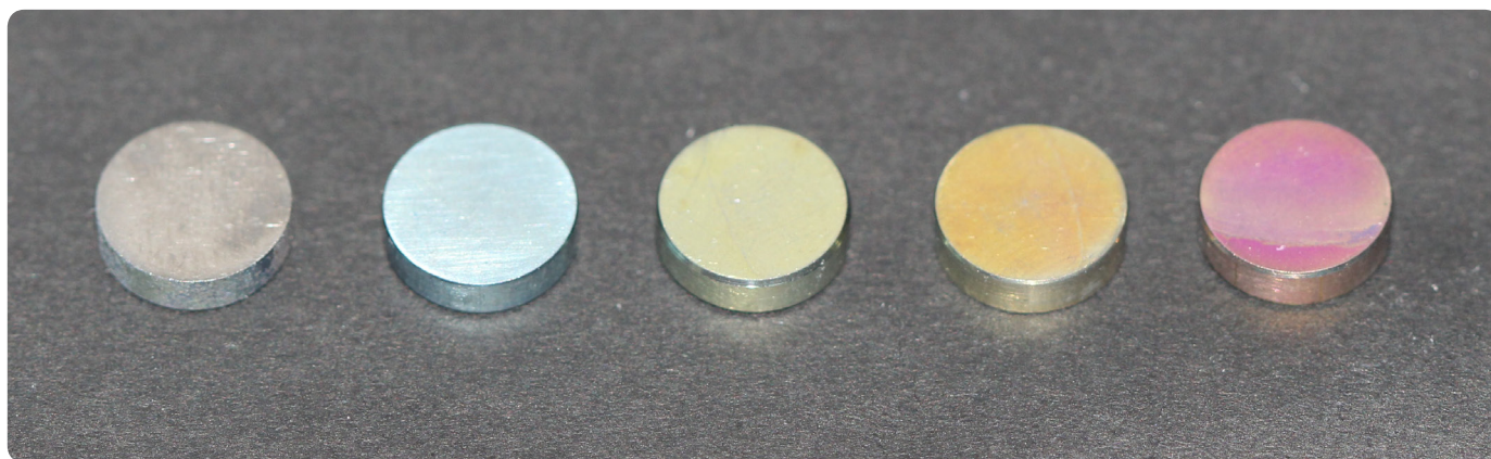
Figure 1: Untreated titanium, 40 V (blue), 50 V (light yellow), 60 V (yellow) and 70 V (pink) anodized titanium (from left to right).
