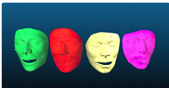
Figure 5: STL meshes of the complete face from all scanners tested. From left to right: Reference STL, RayFace100 STL, Einscan STL and Proface STL.
