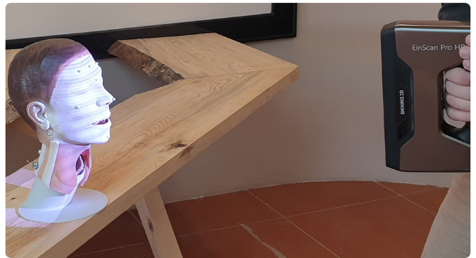
Figure 2: Mannequin head scanned with the Einscan Pro HD scanner.
