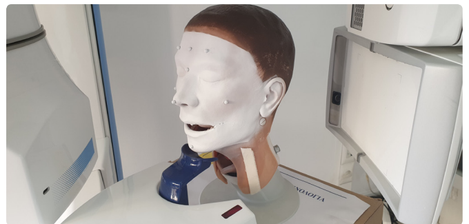
Figure 3: Mannequin head scanned with the Proface 3D Mid scanner.
