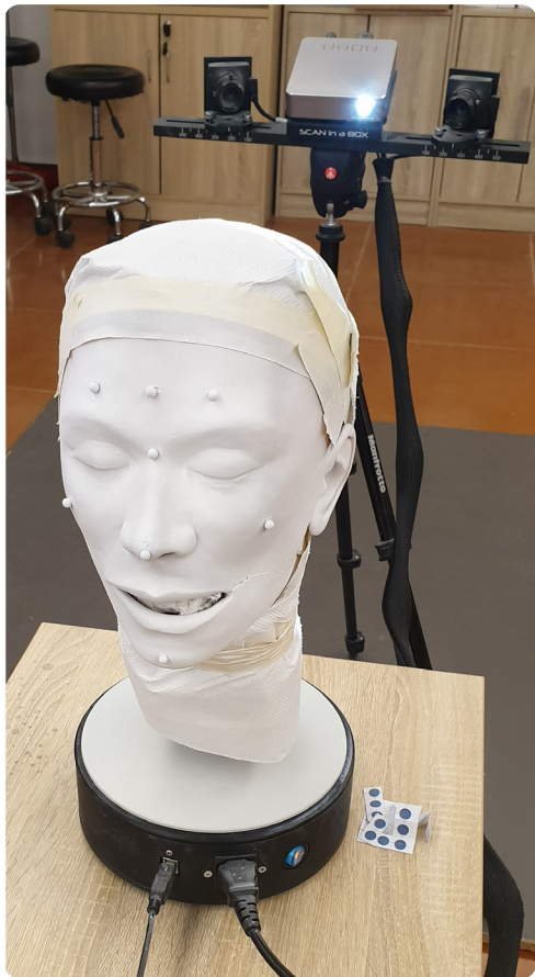
Figure 1: Mannequin head scanned with reference scanner.
