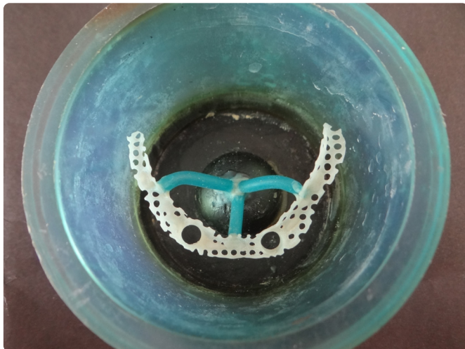
Figure 3: Conventional casting technique used to cast PMMA framework into a Co-Cr framework.
