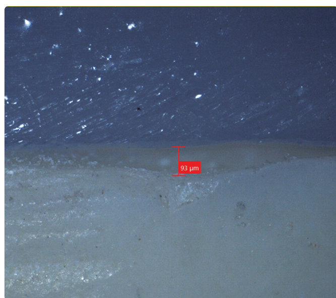
Figure 3: Vertical marginal discrepancy measurement at 200 X magnification.
