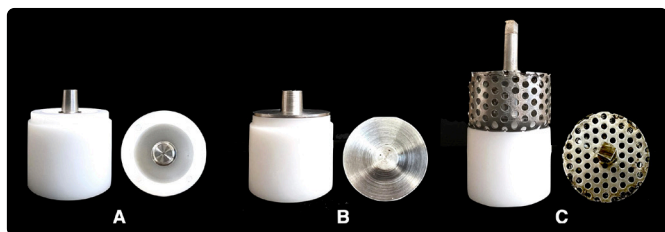
Figure 4: Milled abutment model, cap spacer, and perforated tray. (A) Simulated abutment in plastic block (B) Using cap models covered abutment model as the relieving spacer (C) The abutment model, plastic block, cap spacer, and perforated tray were assembled
