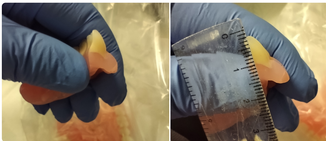
Figure 2: Photos of a fractured 3D printed denture. Note the shear fracture, likely an artifact of the material properties of the denture, despite the acrylic base material thickness measuring 5mm at the point of fracture.
