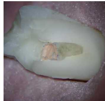
Figure 9 : Unfavourable fracture pattern of Group 2 (Neo spectra ST) [20x magnification in dental operating microscope]
