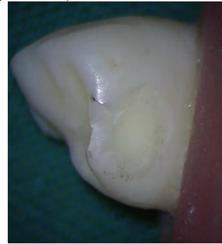
Figure 8: Favourable fracture pattern of Group 1 (control group) [20x magnification in dental operating microscope]
