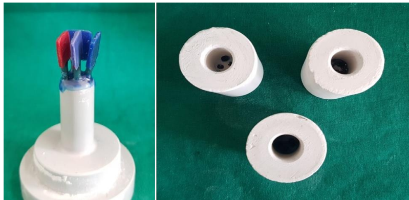
Figure 10: Wax pattern attached to the crucible; invested wax pattern
