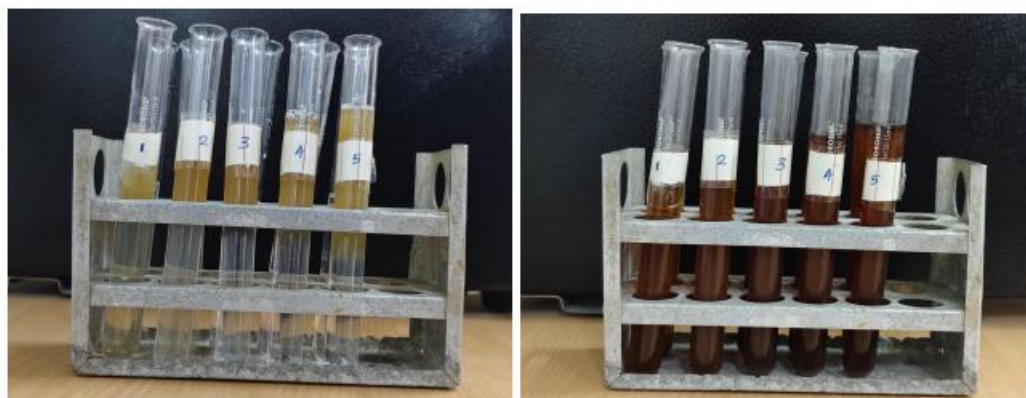
Figure 2 : A. A volume of 100 mL of 1 mM solution of silver nitrate (AgNO 3 ) should be prepared in an Erlenmeyer flask. Add specific volumes of Neem extract (1mg,2mg,3mg,4mg,5mg/ml) to 10 ml of AgNO 3 solution in 20 test tubes. Incubate it for 24 hrs at 37°C in dark chamber . B. Post incubation colour change indicates presence of Silver nano particle
