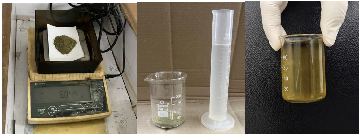
Figure 1: A.5 g of dried neem leaf weighed B.Mixed with 100 ml of Distilled water C. Incubated in dark room at 37°C for 48 hrs.
