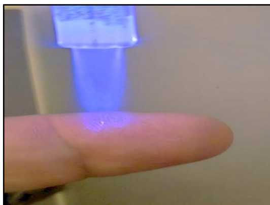
Fig. 8. A photo showing cold atmospheric plasma jet impacting onto cutaneous human layer, indicating the non-thermal identity of plasma discharge.
