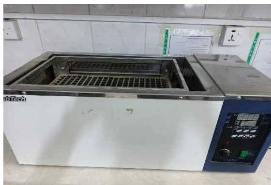
Fig. 5. Ultrasonic bath employed for the detachment of adhered bacteria from the surface of inert polymer granules
