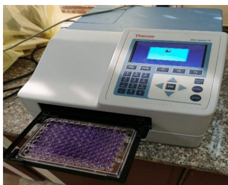
Fig. 7. Thermo Scientific Multiskan FC microplate reader used for the quantitative assessment of biofilm density via optical density (OD) measurement of crystal violet-stained samples.
