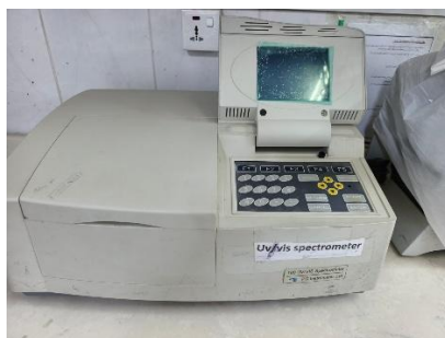
Fig. 6. UV-Vis spectrophotometer used to read the OD of suspensions in order to assess the degree of adhesion (OD).
