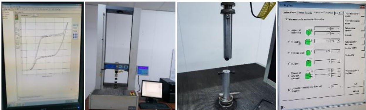
Fig. 4. A. Tensile machine (Lloyd Instrument EZ 20). B. Fit the arch wire into the grips. C. Adjustment of the test setting. D. Stress-strain curve of the NiTi arch wire.
