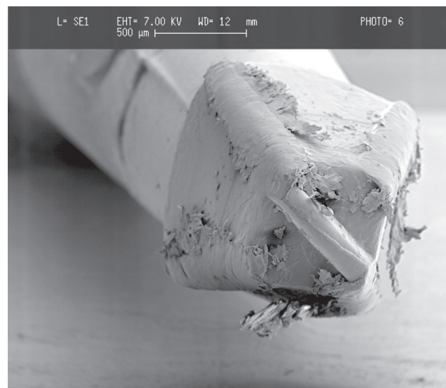
Figure 3. Dulled blades of the used Smartprep™ bur
