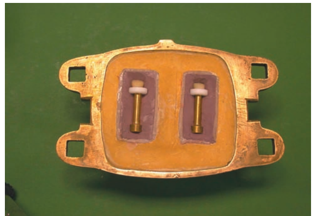
Figure 2. One half of the flask containing the tooth, PTFE collar and brass pattern. These may now be removed, tooth and collar replaced and the mould packed with acrylic resin.
