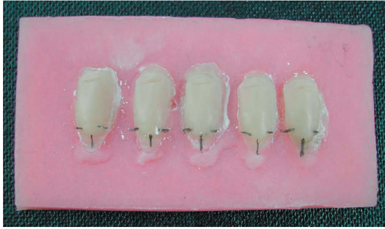
Figure 1. Composite specimens. The specimens were marked to ensure reproducibility of placement of the clasp specimens.
