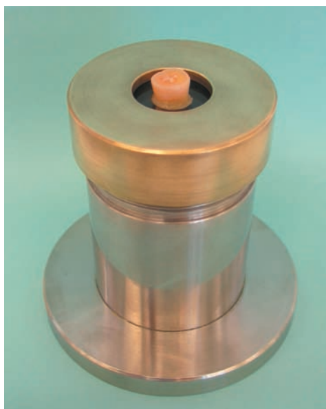
Figure 2. The molar in the test apparatus. The occlusal surface is ground and the roots are in isotonic saline.
