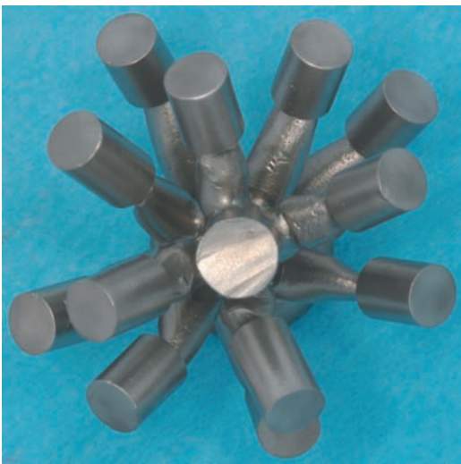
Figure 1. Nickel chrome cylinders prior to sectioning from the sprues
