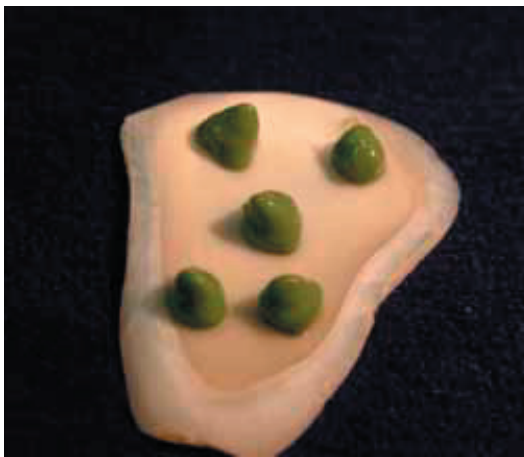
Figure 1. Five impression material specimens on bovine tooth slice.
