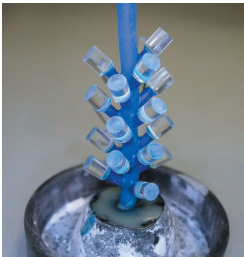
Figure 2. Cylindrical plastic sticks cut into 5mm length, sprued prior to investing
