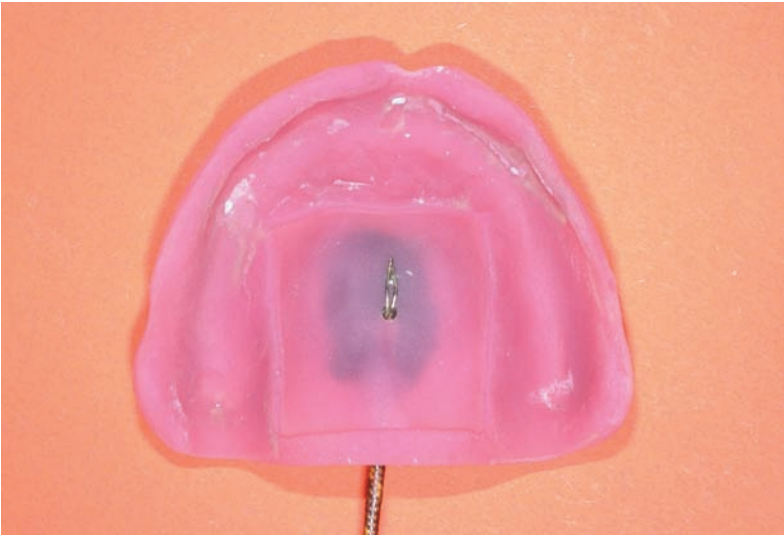
Photo 1. Baseplate with relining area and the thermocouple wire.
