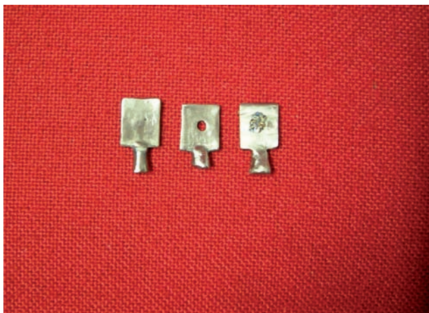
Figure 1. The control group, specimen with perforation and laser welded specimen
