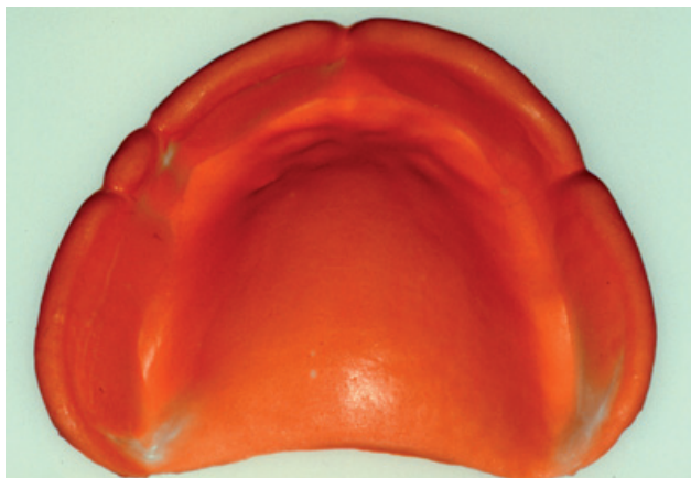
Figure 2. An impression-wafer of the interface space representing the extent of the fit discrepancy of a test denture base.
