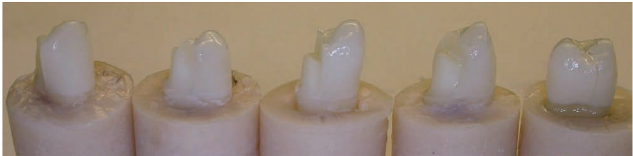
Figure 6. Mode II and mode III Cerec® crown fractures
