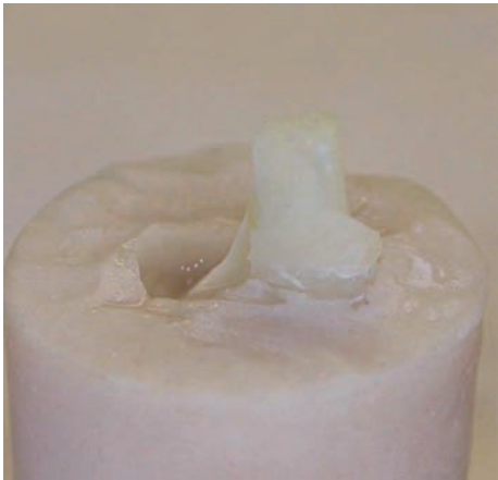
Figure 9. Mode VI catastrophic fracture of Cerec® crown
