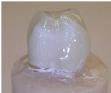
Figure 7. Mode II Lava™ crown fracture
