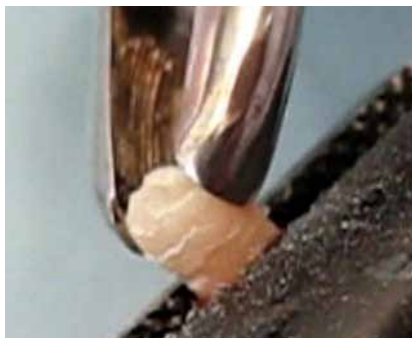
Figure 2. Breaking the core using a sterile pair of forceps
