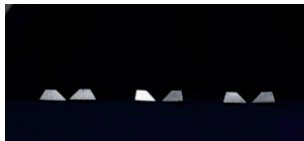
Figure 1. Simulated ridge pairs with outer slopes of 85, 75 and 60 degrees from left to right respectively. Inner slope is 45 degrees for all three ridge types.
