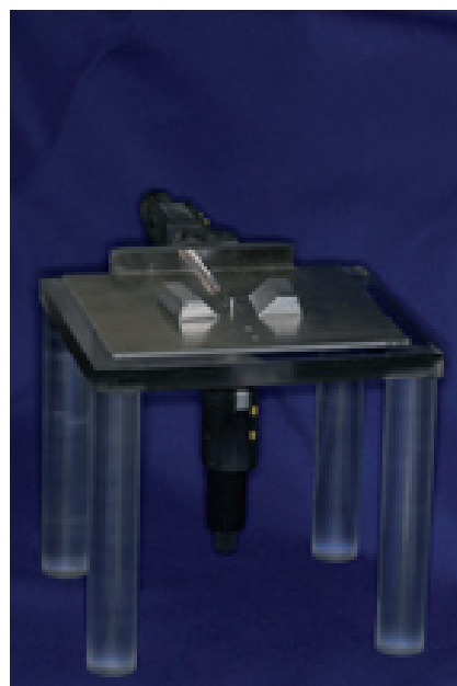
Figure 3. Apparatus used to measure fit of acrylic record base. Vertical micrometer reads distance between intaglio of record base and aluminium plate. The horizontal micrometer displaces the record base in anterior sagittal increments of 1 mm.
