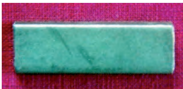
Figure 1. Titanium specimen. Dimension – 26 mm length x 7 mm width x 3mm thickness
