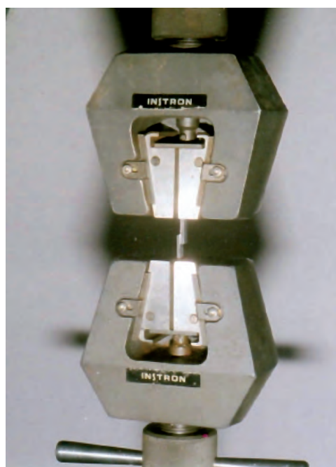
Figure 9. Specimen held in universal testing machine (INSTRON) to detect the bond strength
