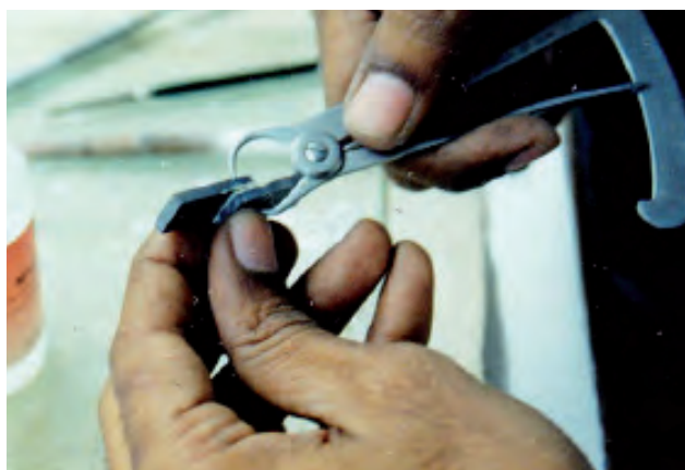
Figure 8. Measuring the thickness of porcelain in between two titanium specimens using Iwanson's gauge
