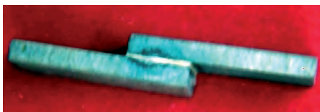
Figure 7. Titanium – Porcelain sandwich (after porcelain firing)
