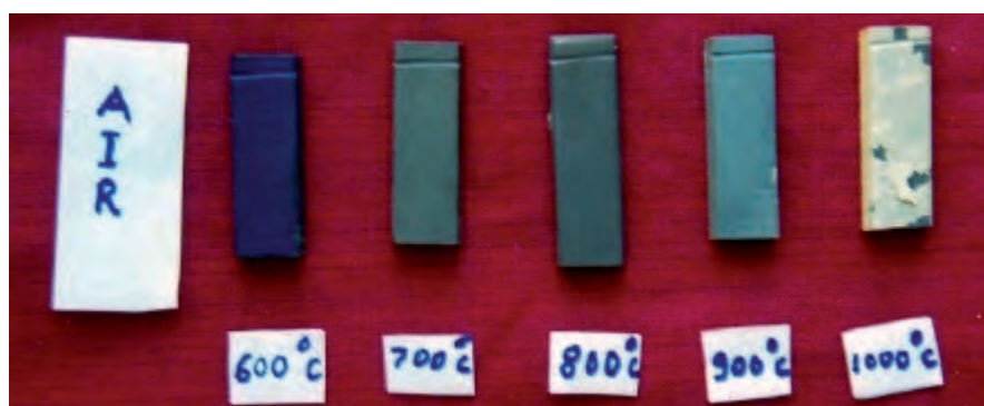
Figure 4. Preoxidation of Titanium specimens under air at various temperatures
