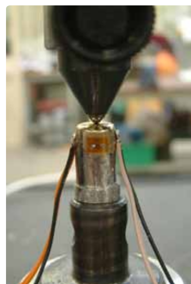
Graph 2: Cemented sample under compressive loading.
