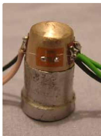
Graph 1: Strain gauge on the axial surface and another on the Opposing surface (1mm above the crown margin).
