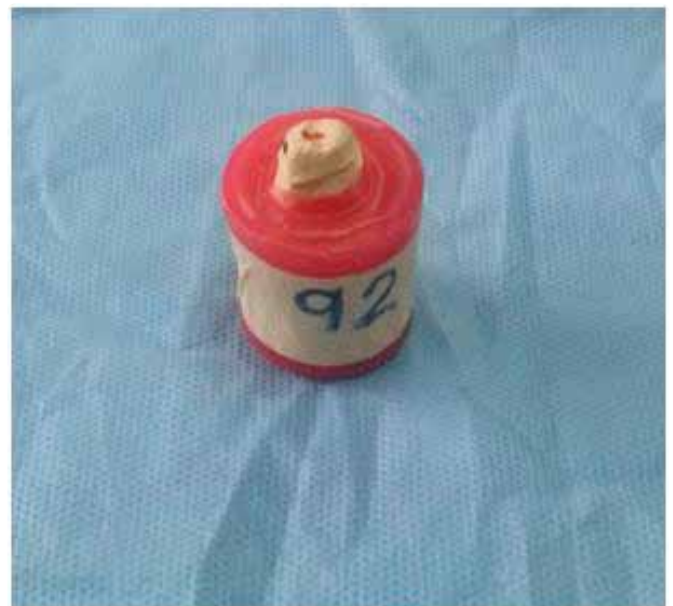
Figure 1: Anterior view of the die fixed in the center of wax cylinder.
