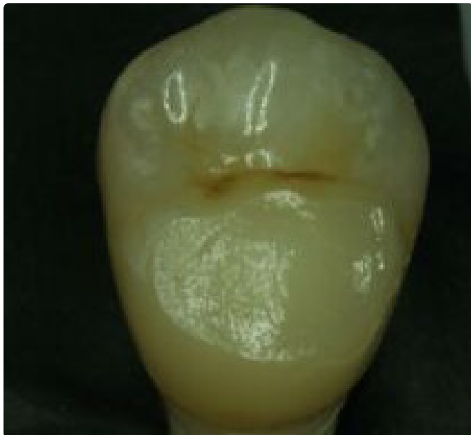
Figure 2: Chipping of the veneering of the zirconia/ ceramic during TCML but no zirconia exposition was visible.
