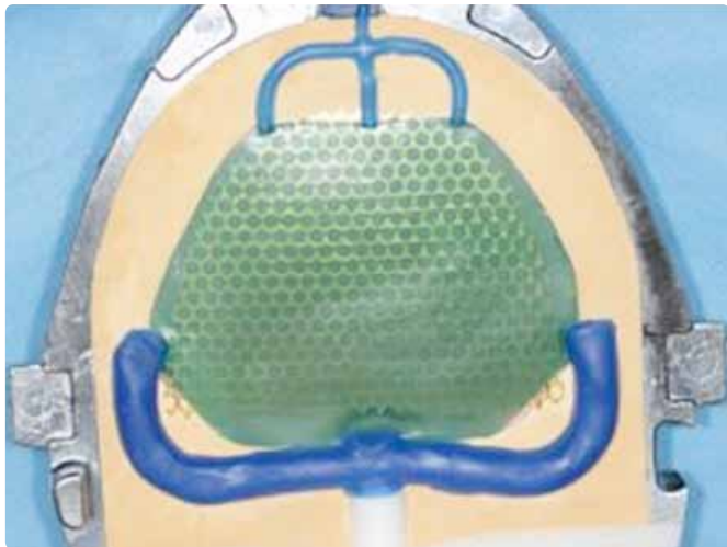
Figure 1: Wax/grit strengthener plate in injection molding flask with sprues. Arrows show reposition area without wax covering the grid.
