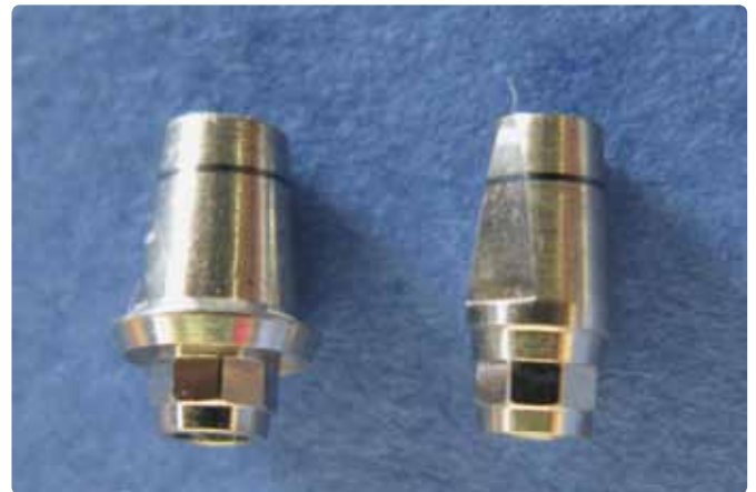
Figure 2: The abutments of two groups. Left, abutment with finishing line on it (abutment-level specimen). Right, abutment without finishing line for crown margin placement (implant-level specimen).
