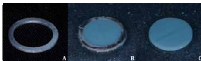
Figure 2: Cylindrical aluminum matrix used to framework standardization. (A) Cylindrical aluminum matrix, (B) liquefied wax into the matrix, (C) solid wax disc after matrix removal.
