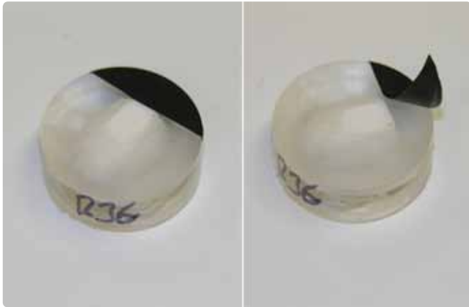
Figure 1: Insulation tape placed across the acrylic reference area to protect against toothbrush abrasion.
