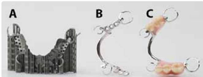
Figure 2: RPD Co-Cr framework with support structures after SLM B. Support structures removed and finishing accomplished in the same manner as standard conventionally manufactured Co-Cr frameworks C. Finished Co-Cr RPD framework. Source: EOS GmbH
