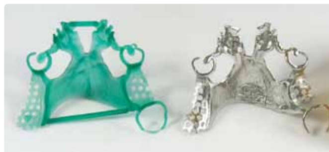
Figure 1: 3D-printed resin and cast Co-Cr RPD frameworks. Source: 3D Systems
