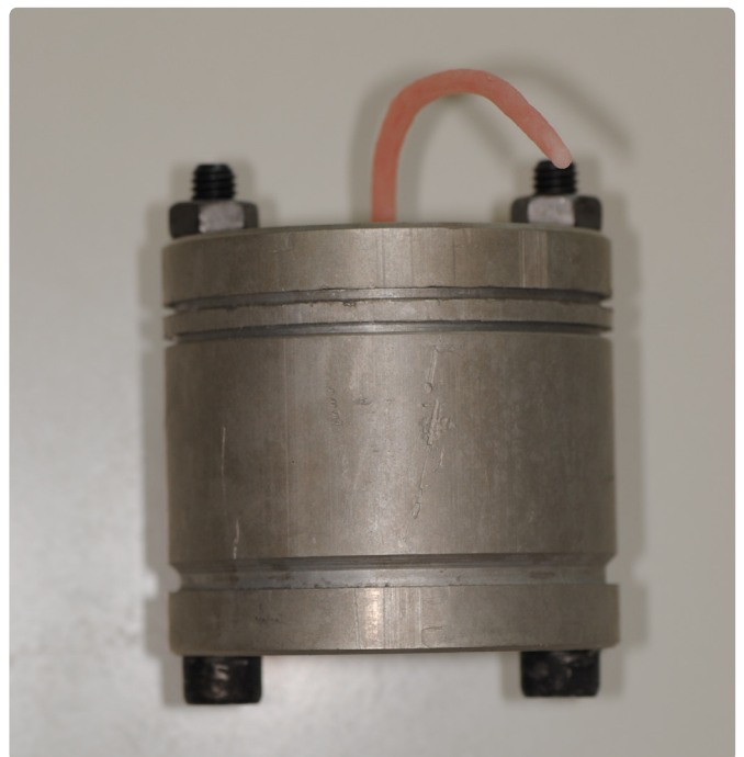
Figure 4: A mold assembled during the packing process.
