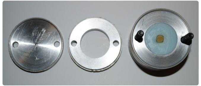
Figure 2: An acrylic denture tooth placed in silicone, with only the ridge lap surface accessible.
