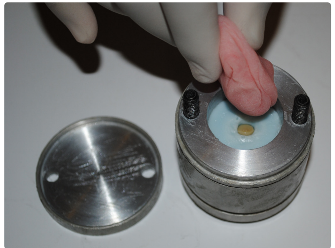
Figure 3: PMMA acrylic resin packing.
