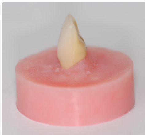
Figure 5: An acrylic denture tooth with the corresponding PMMA resin base after the polymerization process.
