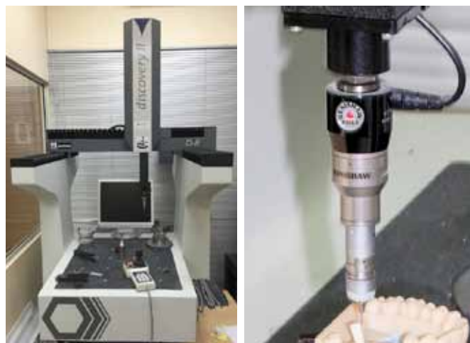
Figure 1b and c: The measurement of the implant features for each model was completed using a Sheffield Discovery II D-8 Coordinate Measuring Machine (CMM). As shown in Figure 3 the CMM was fitted with a Probing System comprising a Renishaw PH6A Probe Head, TP20 Medium Force Body and a \varnothing 1mm Stylus.
