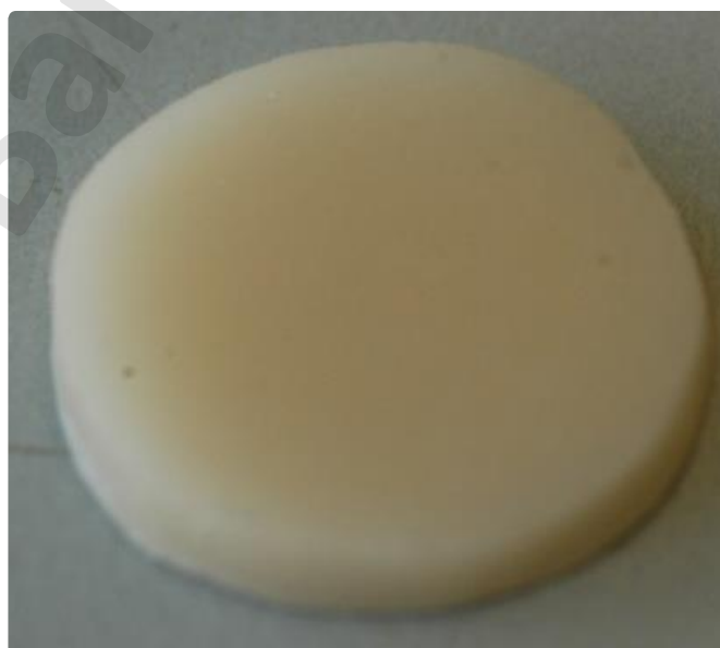
Figure 1b: Composite disc produced using the PVS mould
