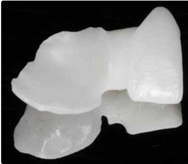
Figure 1: Anterior YTZP ceramic RBB framework following CAD-CAM manufacturing and before the addition of veneering material.
