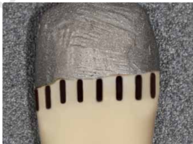
Figure 2: For marginal gap measurement, predefined measuring points on typodont master model with representative metal coping
