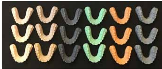
Figure 2: For each printer, 3 dentate models (DMs) were printed with the material indicated by the producer. These DMs were cured and kept for a period of 1 month in a dark box, away from any heat source; after this period of time, they were scanned with a desktop scanner (Freedom UHD®). The standard tessellation language (STL) files obtained from this process were then imported into a reverse engineering software (Studio 2012®) and superimposed on the original reference model, to investigate trueness and stability over time.
