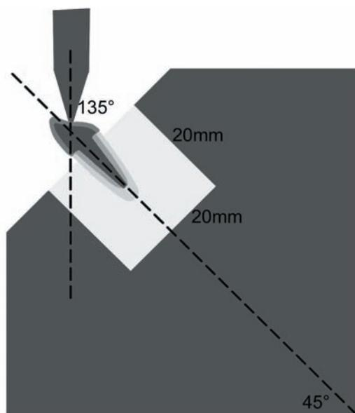
**Figure 3.** Diagrammatic representation of the method used for fracture strength testing.
