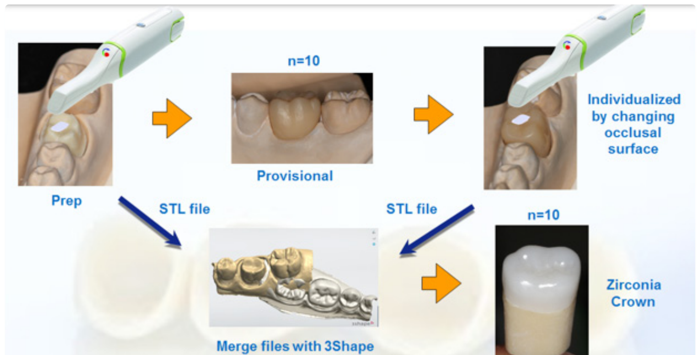
Figure 1: Experimental design 1. Manufacturing the temporary and permanent FDPs: Using a E4D scanner, Telio Cad Temporary FDPs (PMMA) were made and their occlusion adjusted individually. Afterwards the PMMA crowns were scanned and the anatomy of the crowns inserted into the scan of the crown preparation. The resulting .stl-file was used to produce Zir-CAD LT (ZrO 2 ) crowns.
